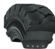
Resilient Solid Tyre Sectional View
